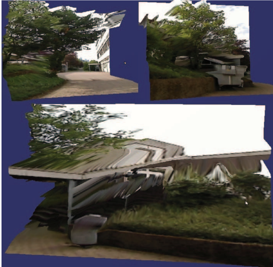
Figure 2.3: Examples of 2D-3D mapping between LIDAR and Camera [13]
